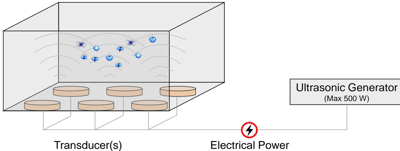
“Power” often refers to the **Electrical Power [W]** from the generator delivered to the transducers. Some vendors offer a “Watt Meter” to measure this. This does not account for the transducer efficiency.
