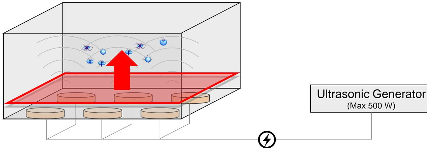
Measuring the **Acoustic Power [W]** is valid only when sound waves propagate in one direction (i.e., no reflections from surface or side walls), which is NOT the case for most cleaning tanks. The **Acoustic Power** should account for the total radiating area. If transducers are mounted across the bottom of the tank, the area can be estimated from the bottom surface dimensions of the tank.
