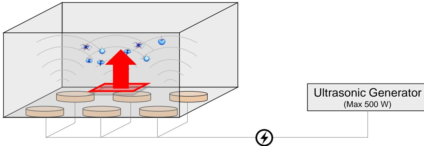
The same issues apply when measuring the **Acoustic Intensity** [ $\text{W}/\text{cm}^2$ ], which is defined by the acoustic power over a defined radiating area in the direction perpendicular to that area. It should be noted that the acoustic field is typically NOT uniform.
