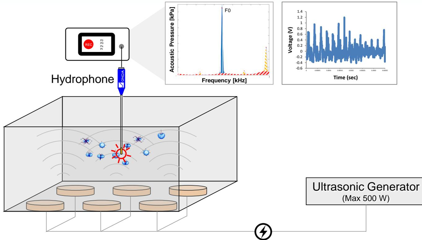
Most hydrophones are based on a piezoelectric transducer that generates an electrical signal or a **Voltage [V]** when subjected to a change in **Acoustic Pressure [kPa]**. Ideal hydrophone designs enable measurements to be sensitive from all directions at a single point. Hydrophone calibrations enable measurements of absolute **Acoustic Pressure**. Pressure is the unit of measure most representative of what “cleans” parts.
